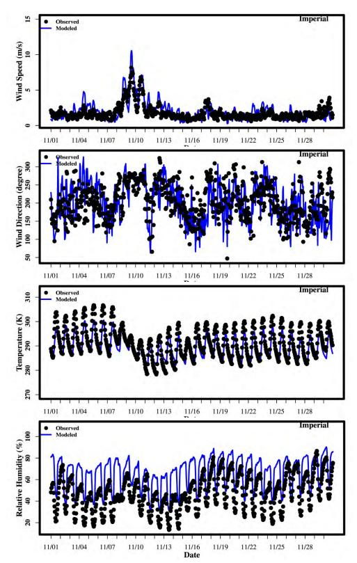
Figure S. 11 Time series of wind speed, direction, temperature and relative humidity for Imperial County in November 2012.
