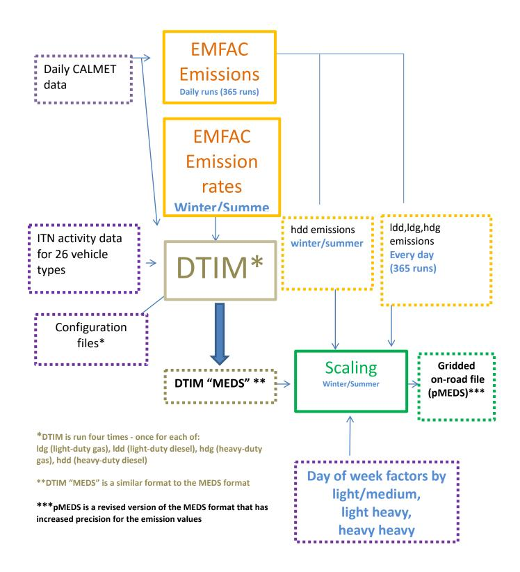
Figure 3 Block diagram for on-road processing
