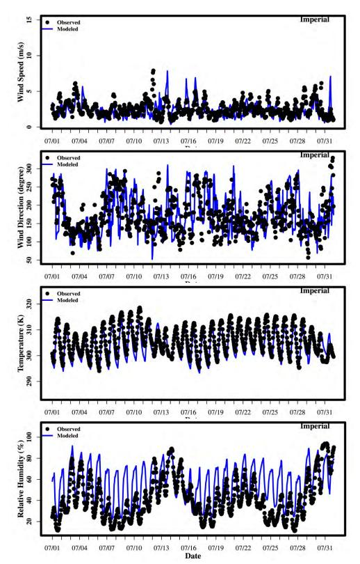
Figure S. 7 Time series of wind speed, direction, temperature and relative humidity for Imperial County in July 2012.
