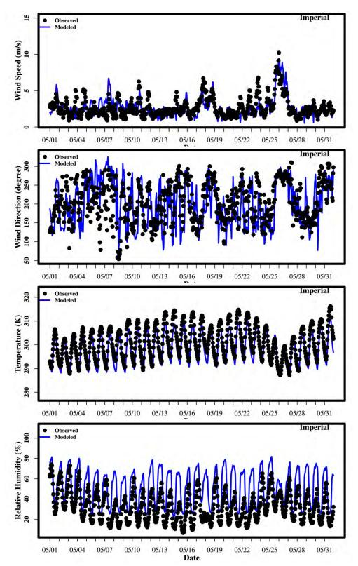
Figure S. 5 Time series of wind speed, direction, temperature and relative humidity for Imperial County in May 2012.
