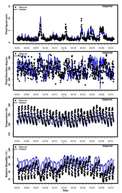
Figure S. 1 Time series of wind speed, direction, temperature and relative humidity for Imperial County in January 2012.
