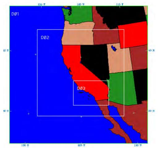
Figure 1. WRF modeling domains (D01 36-km; D02 12-km; and D03 4-km).
