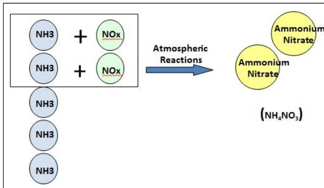
**Figure 3.3 Reducing the less abundant precursor is more effective in reducing Ammonium Nitrate**
