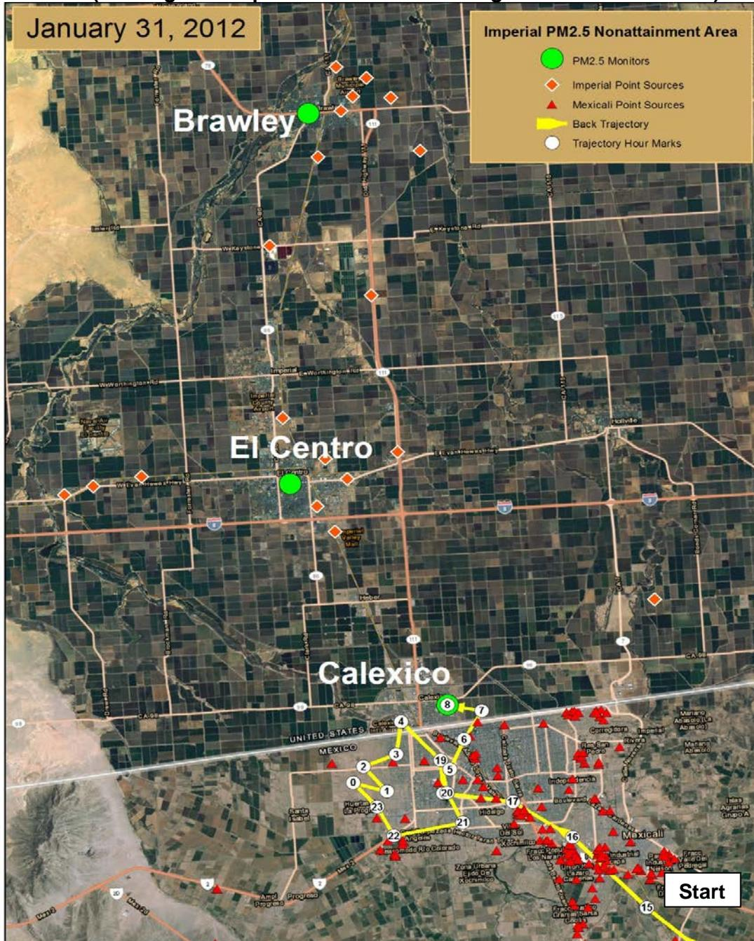
The back trajectory developed for January 31, 2012 started at Calexico at the hour of the highest PM<sub>2.5</sub> BAM concentration (8:00 am) and followed an air parcel back to
