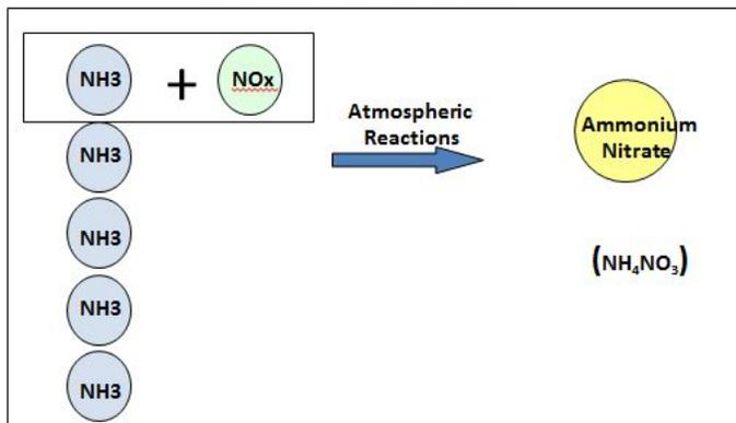
**Figure 3.4 Reducing the more abundant precursor is less effective in reducing Ammonium Nitrate**
